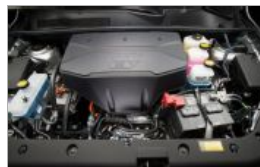
Although the RAV4 EV's "engine cover" says Toyota, the motor is actually a detuned Tesla Model S unit.
